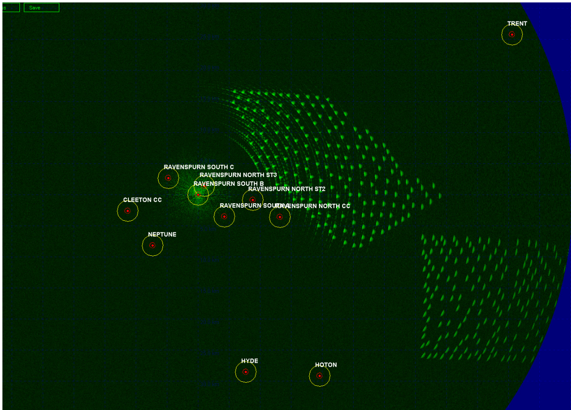
Figure 23: Ravenspurn South B platform REWS clutter map showing returns from the turbines and sea clutter from the cumulative Hornsea projects.
